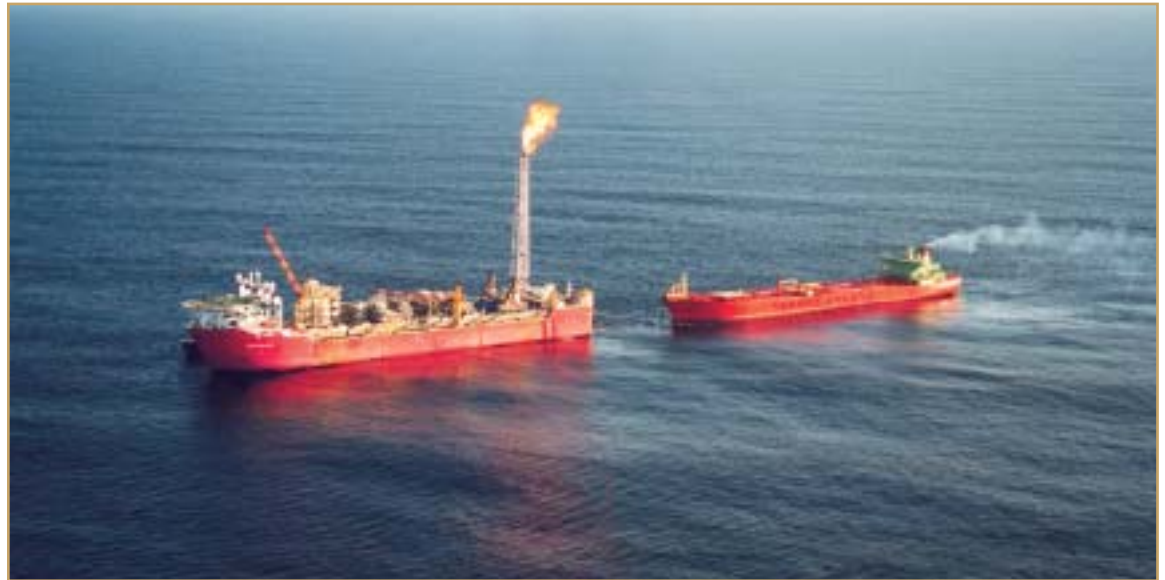
Credit: Terra Nova Oil tanker receiving oil from the Terra Nova Floating Production, Storage and Offloading vessel
